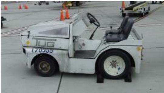
**Figure 1 - Correctly chocked vehicle**
