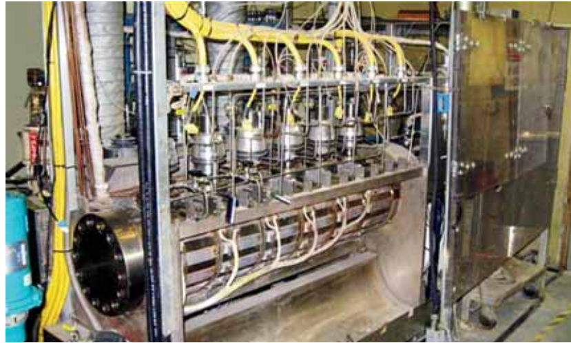
Ore from Lagunas Norte in Peru will undergo metallurgical test work in this scale pressure oxidation circuit at the Barrick Technology Center as part of the prefeasibility study expected to be completed by the end of 2012.
